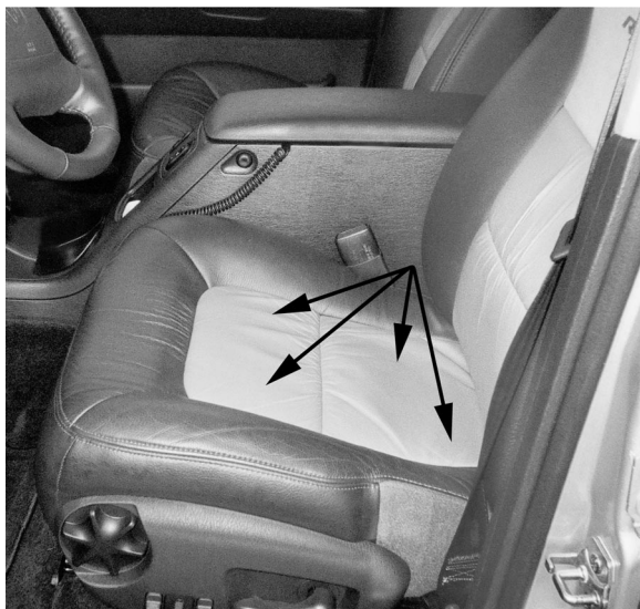
Figure 2. Picture of the car seat with arrows pointing at the location of the heating coils that caused this patient's burn injury at 120°F.
