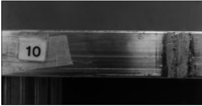
Fig. 2a Loosely Tied Ladder Flange Damage
