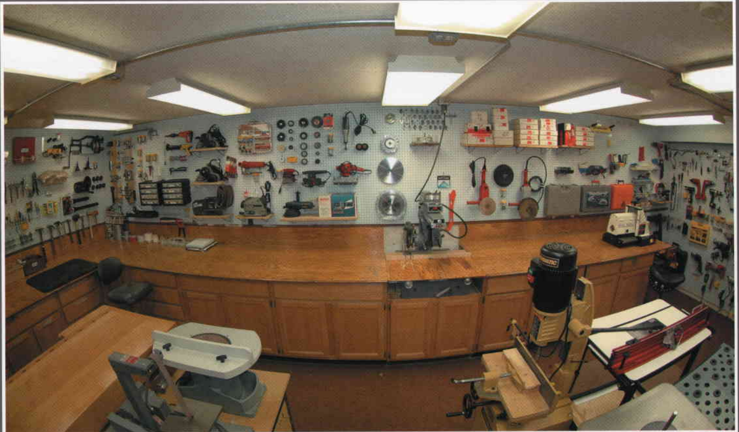
Figure 6 - 12" Radial Saw with ripping capability (center). Portable Sanding Machines on the wall have equivalent stationary machines in the island. You can drill a square hole with a Mortising Machine (right front).
