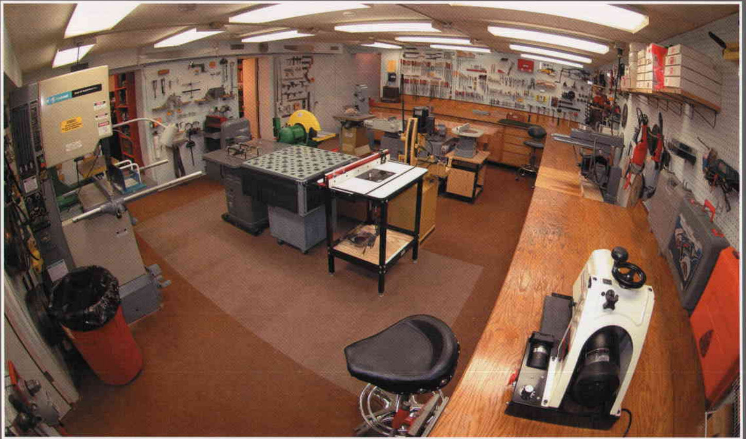
Figure 3 - Shaper, Vacuum Table, Router Table (center).
