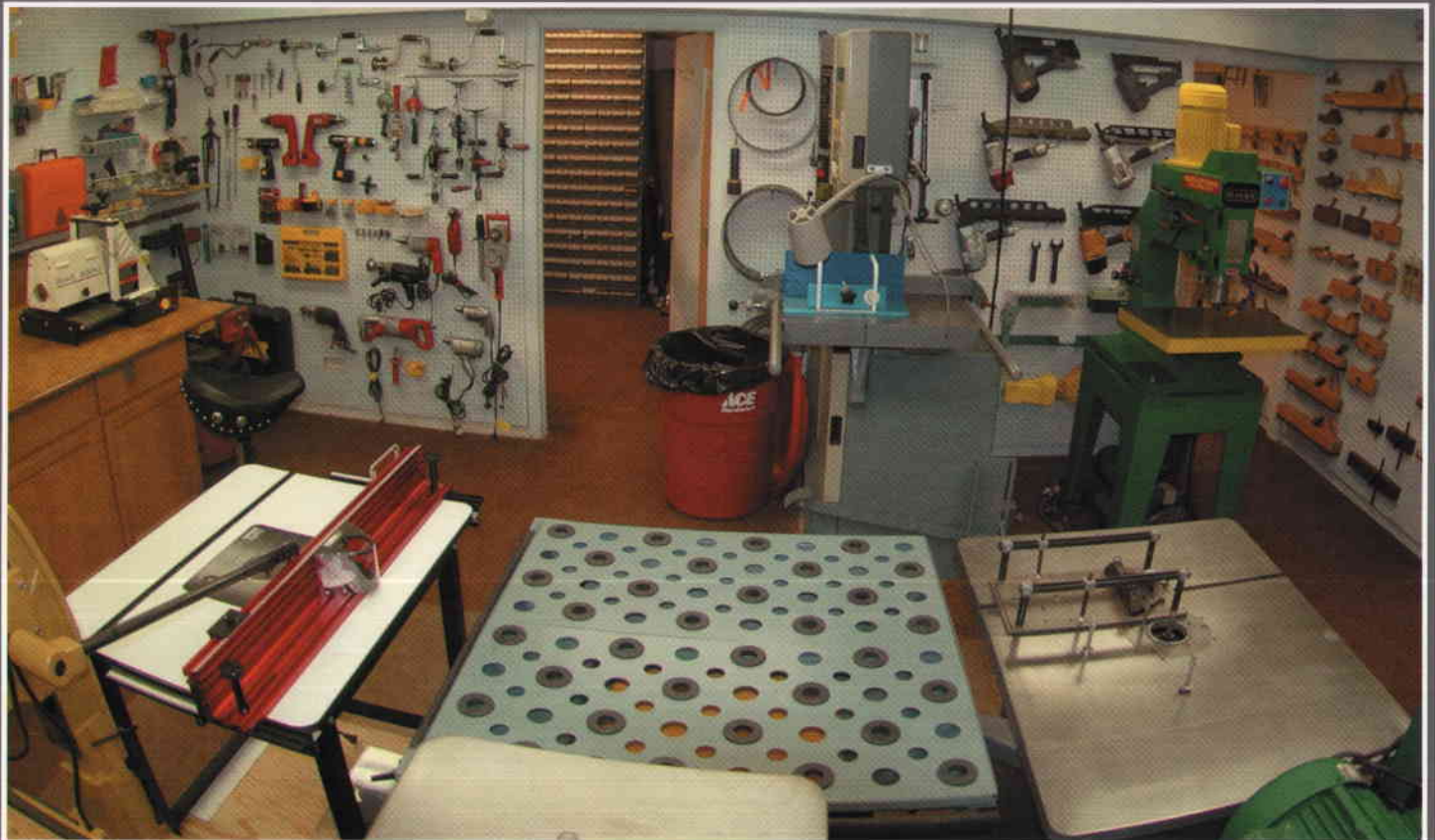
Figure 4 - Six Braces, Three Hand Drills, Four Breast Drills, Four Battery Powered Hand Drills, Seven Electric Drills, Two Hammer Drills, Push Drills (left rear wall). 20" Metal / Wood Bandsaw (center rear). Overhead Router (right rear). Six Nail Guns (center rear wall).
