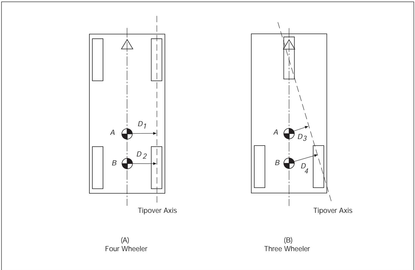
Figure 7. Effects of vehicle loading on four- and three-wheeled vehicles
