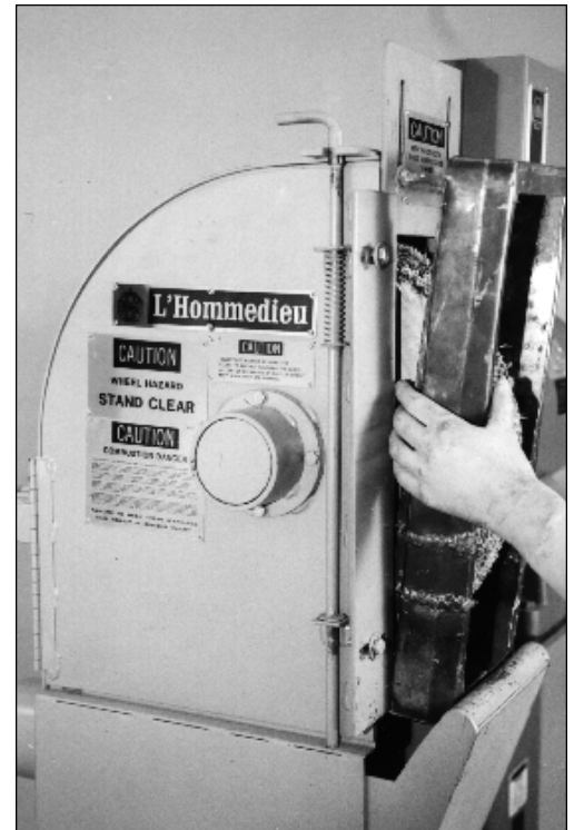
Figure 12. Entrapment between workpiece and hood.
