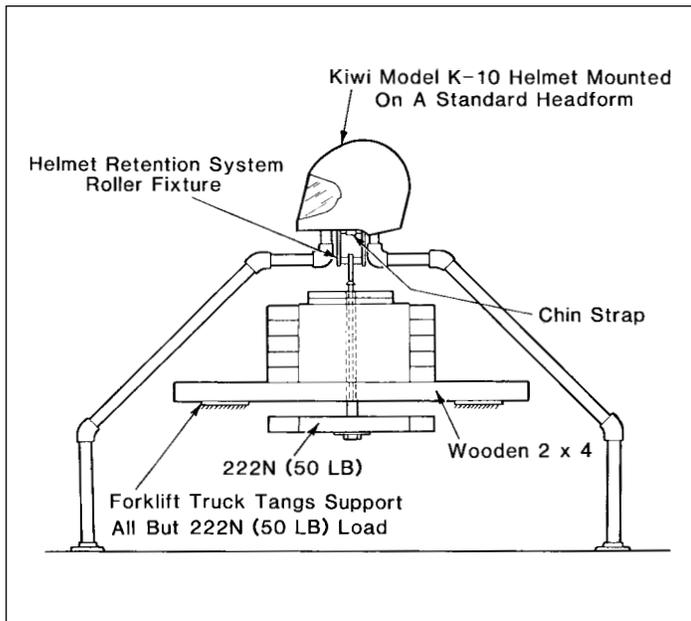
Figure 2. Helmet Retention System Preloading Apparatus
