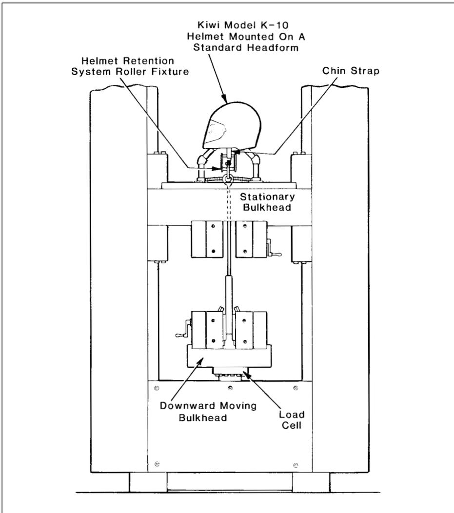
Figure 4. Helmet Retention System Apparatus for Loading to Failure
