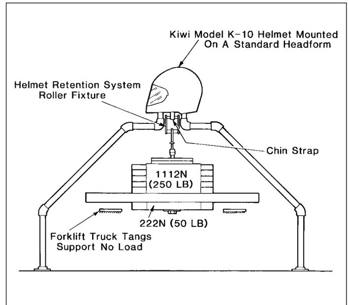
Figure 3. Helmet Retention System Testing Apparatus
