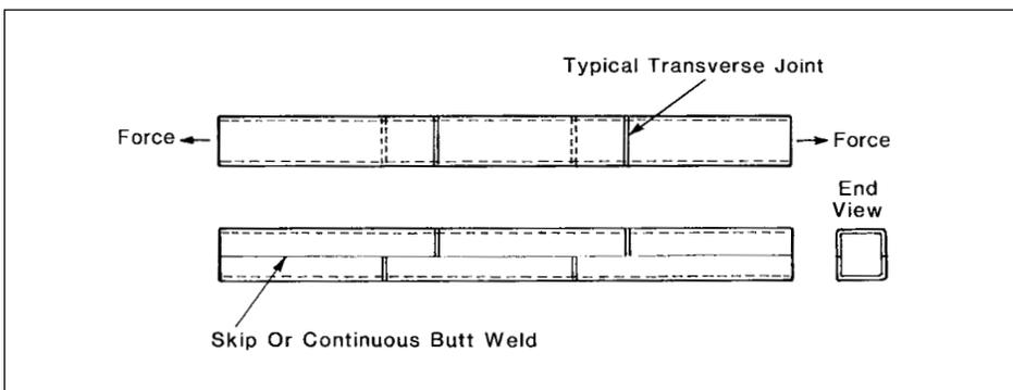
Figure 5. Tensile Box Element - No Transverse Welds
