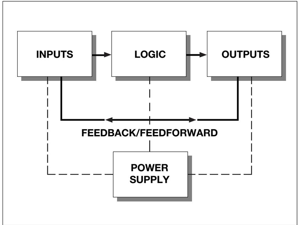
Figure 1. General Control System Block Diagram
